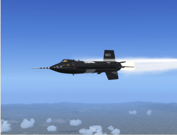
X-15-1 for Flight Simulator with the XLR-11 engines and the NACA “vane-type” boom nose. This is the limited-mission configuration.
