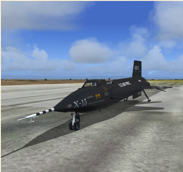
X-15-1 for Flight Simulator (rollout version), sporting the NACA "vane-type" boom nose.
