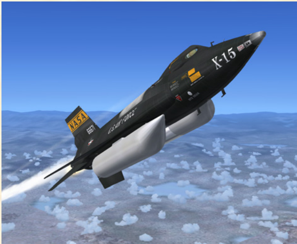
X-15A-2 for Flight Simulator. Note the external propellant tanks.
