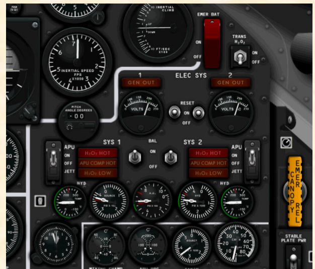
A closer view of the electrical section on the X-15-1 main instrument panel. Note the APU and generator switches and the AC bus voltmeters.
