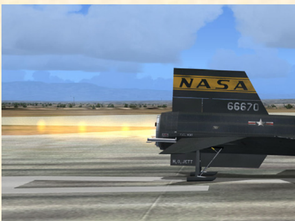
XLR-99 engine start on the X-15-1 for Flight Simulator. The XLR-99 engine produced nearly 60,000 pounds of thrust at high altitude.
