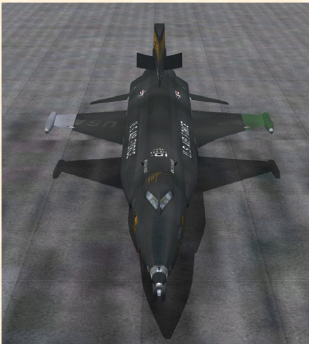
X-15-1 in her design-mission configuration. Note the ball nose, the ballistic control system rockets and the open speed brakes at the rear. This aircraft also carries wing-tip pods covered with gray and green thermopaint.
