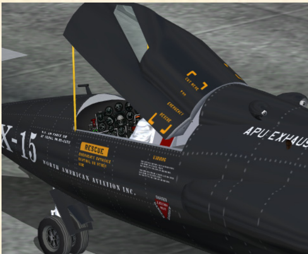
X-15-1 (limited-mission configuration) showing the main instrument panel inside the cockpit.
