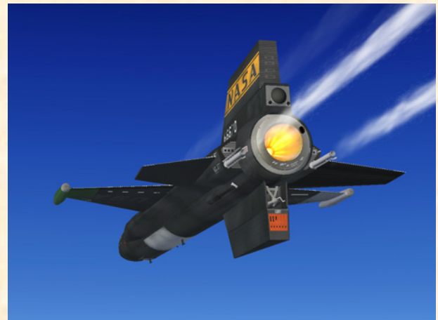
X-15-1 for Flight Simulator (XLR-99 engine). Note the flames inside the engine nozzle (second stage igniter effect) and the flow of liquid oxygen and ammonia coming out of the rear prime drains.
