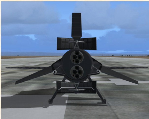
Rear view of the X-15-1 showing the large split-flap upper and lower speed brakes.
