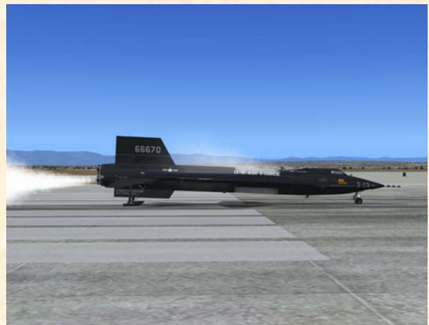
X-15-1 venting her propellant tanks. Frost and condensation from the cold propellants can be seen on the fuselage and around the internal liquid oxygen tank. The boiling point of liquid oxygen is -297^{\circ} F in standard atmospheric conditions.
