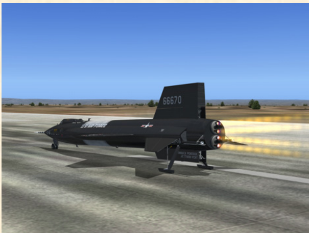
X-15-1 at launch. The upper and lower XLR-11 engine thrust chambers are ignited in sequence.
