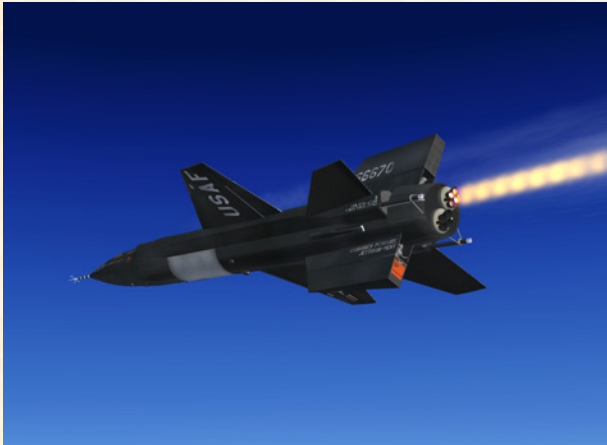
Reaction Motors XLR-11 liquid-fuel rocket engines on the X-15-1 for Flight Simulator. Note that the number 2 engine has been shut down.
