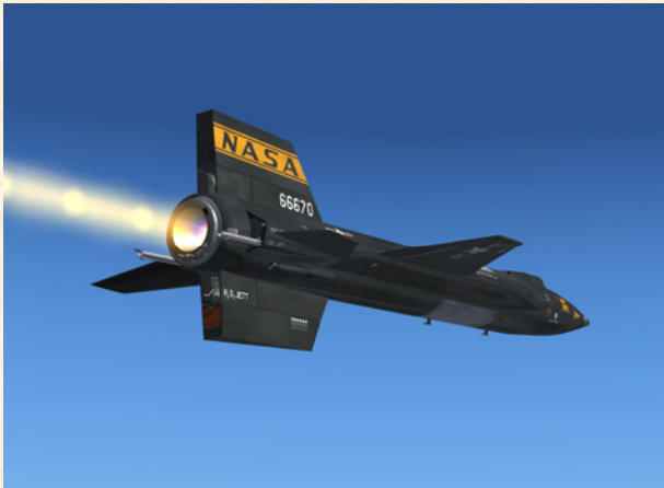
The million-horsepower Reaction Motors XLR-99 engine on the X-15-1 for Flight Simulator. The XLR-99 was a liquid-fuel turbo-rocket engine of variable-thrust design capable of delivering up to 60,000 pounds of thrust at high altitude.
