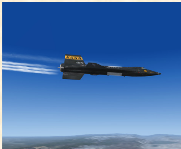
The three propellants (liquid oxygen, ammonia and hydrogen peroxide) are being dumped overboard through the jettison ports at the back of the X-15-1 for Flight Simulator.
