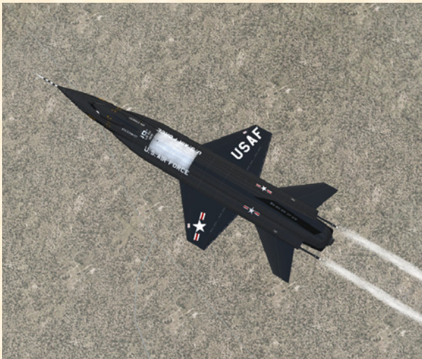
X-15-1 (XLR-11 engines). Note the frost on the fuselage, around the liquid oxygen tank, and the flow of propellants coming out of the rear jettison ports.
