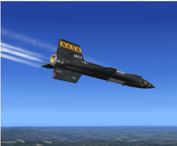
Before landing, the remaining propellants are dumped overboard through the jettison ports on the X-15-1 for Flight Simulator.
