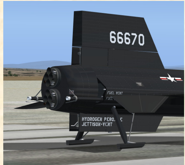
Rear view of the X-15-1 showing the XLR-11 engines. Note how both engines are slightly canted so that their thrust vector intersects at the aircraft's center of gravity for stability reasons. Also, the ventral rudder does not appear on the X-15 at this time to provide ground clearance and enough space for the rear landing skids.
