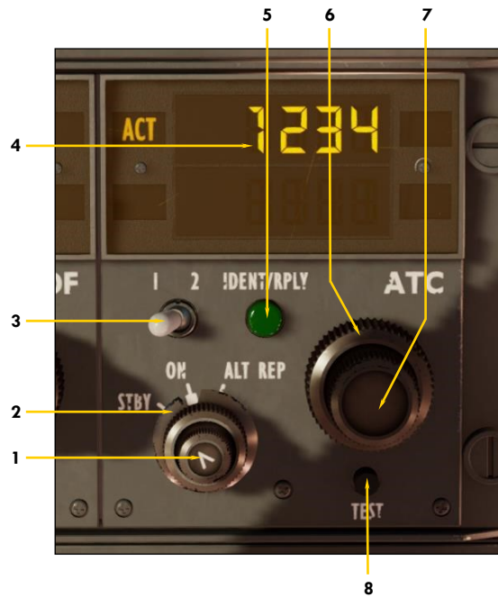
TRANSPONDER (ATC RADIO) Figure 5-21
