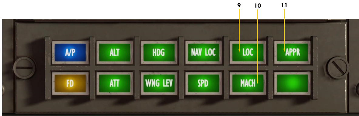
AUTOMATIC FLIGHT CONTROL SYSTEM / AUTOPILOT / FLIGHT DIRECTOR MODE SELECTOR PANEL Figure 5-22b
