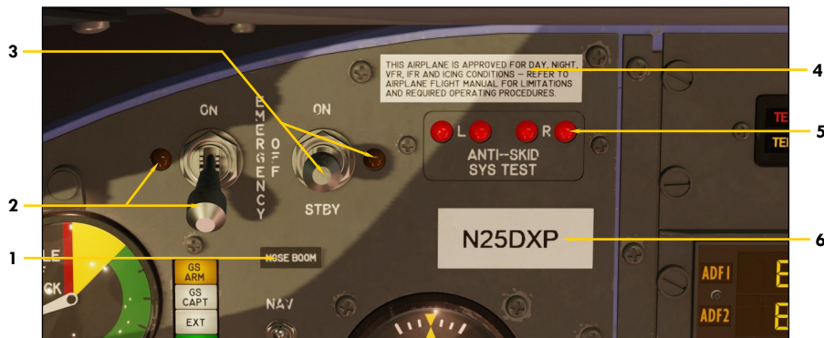
EMERGENCY BATTERY SWITCHES AND ANTI-SKID LIGHTS Figure 5-15
