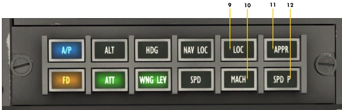
AUTOMATIC FLIGHT CONTROL SYSTEM / AUTOPILOT / FLIGHT DIRECTOR MODE SELECTOR PANEL Figure 4-22d
