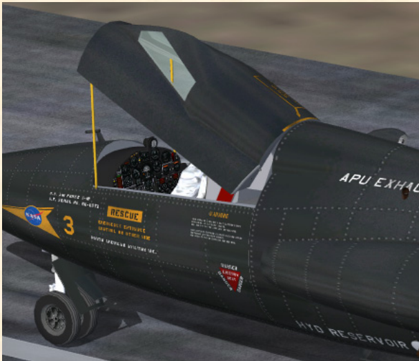
X-15-3 showing the main instrument panel inside the cockpit. Note the upper right bug-eye camera port.
