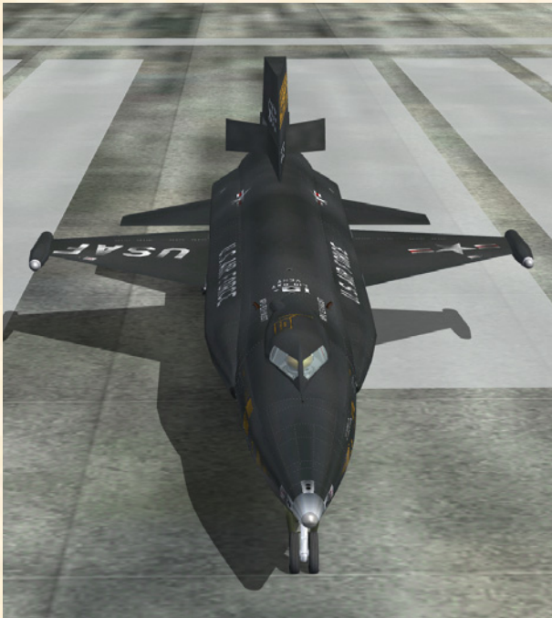
X-15-3 for Flight Simulator. Note the ball nose, the ballistic control system rockets and the open speed brakes at the rear. This aircraft also features wing-tip pods and a tail-cone box with research instruments.
