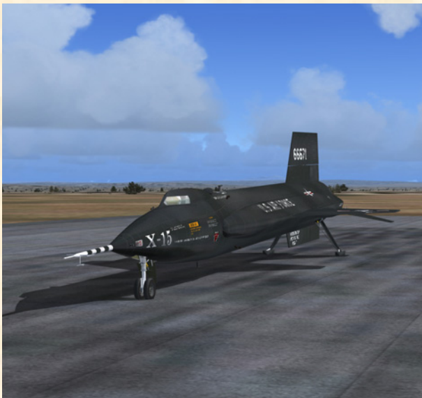
X-15-2 for Flight Simulator, sporting the NACA "vane-type" boom nose.
