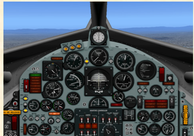
The instrument panels on the X-15-3 were modified and improved in early 1963. The original black panels were replaced by light blue-gray panels which contrasted better with the gauges, light indicators and flight instruments.
