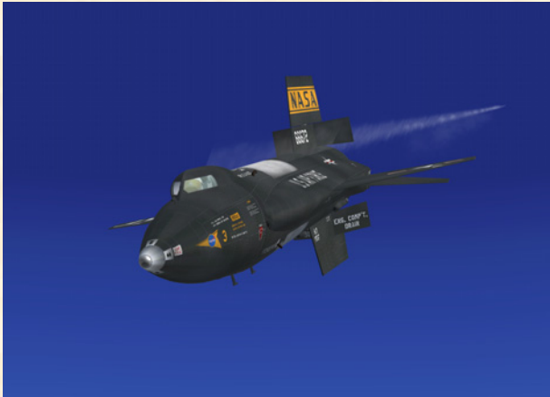
X-15-3 during her descent and about to perform a 5G pullout to level flight at about 65,000 feet.
