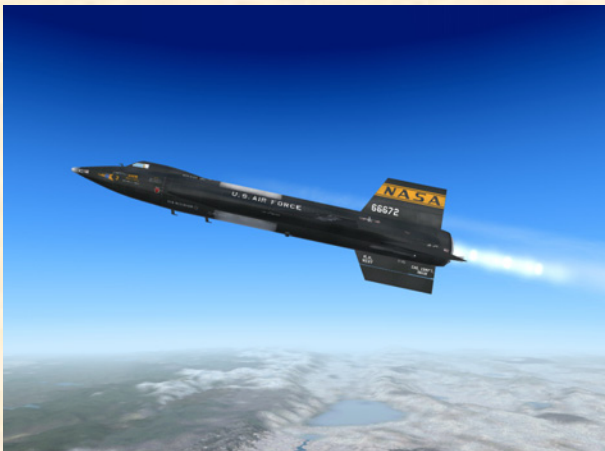
The million-horsepower Reaction Motors XLR-99 engine on the X-15-3 for Flight Simulator. The XLR-99 was a liquid-fuel turbo-rocket engine of variable-thrust design capable of delivering up to 60,000 pounds of thrust at high altitude.
