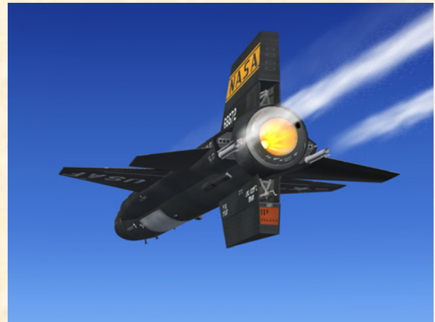
X-15-3 for Flight Simulator (XLR-99 engine). Note the flames inside the engine nozzle (second stage igniter effect) and the flow of liquid oxygen and ammonia coming out of the rear prime drains.
