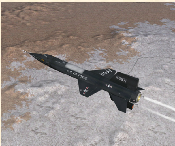
X-15-2 in flight. Note the frost on the fuselage, around the liquid oxygen tank, and the flow of propellants coming out of the rear jettison ports.
