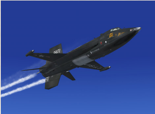
X-15-3 just before launch. Note the flow of ammonia and liquid oxygen coming out from the back of the aircraft during the engine prime phase.
