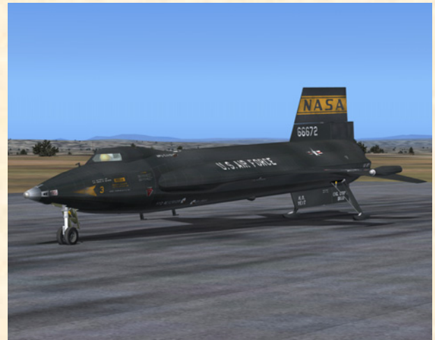
X-15-3 at Edwards AFB. Note the dual wheel front gear and the two rear landing skids. The blue NASA insignia on the front side and some other markings have burned off during multiple reentries into the earth's atmosphere.
