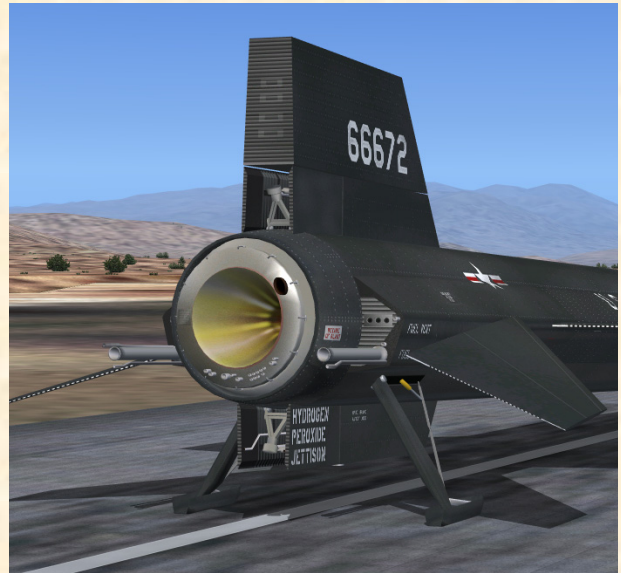
Rear view of the X-15-3 showing the XLR-99 rocket engine. The ventral rudder does not appear on the X-15 at this time to provide ground clearance and enough space for the rear landing skids.
