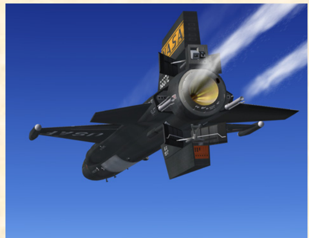
XLR-99 engine installed on the X-15-3 (design-mission configuration). Note the open speed brakes.
