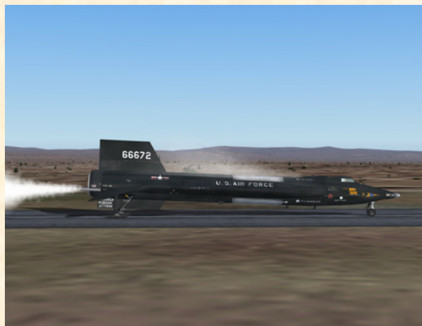
X-15-3 venting her propellant tanks. Frost and condensation from the cold propellants can be seen on the fuselage and around the internal liquid oxygen tank. The boiling point of liquid oxygen is -297^{\circ} F in standard atmospheric conditions.
