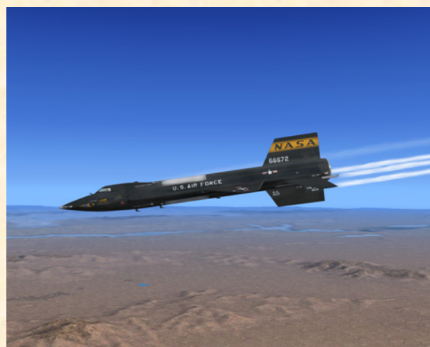
The three propellants (liquid oxygen, ammonia and hydrogen peroxide) are being dumped overboard through the jettison ports at the back of the X-15-3 for Flight Simulator.
