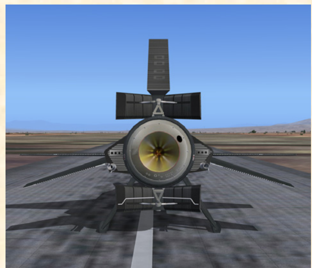
Rear view of the X-15-3 showing the large split-flap upper and lower speed brakes.
