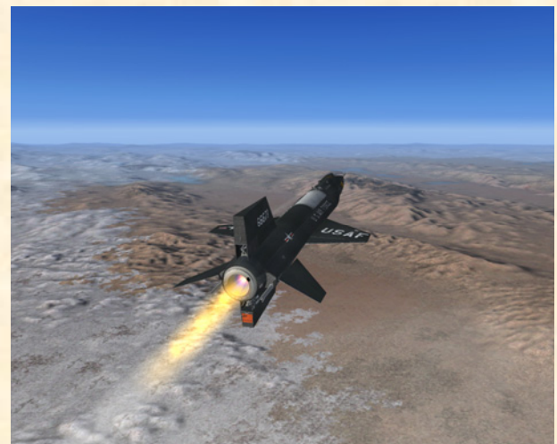
XLR-99 engine start on the X-15-2 for Flight Simulator. The XLR-99 engine produced nearly 60,000 pounds of thrust at high altitude.
