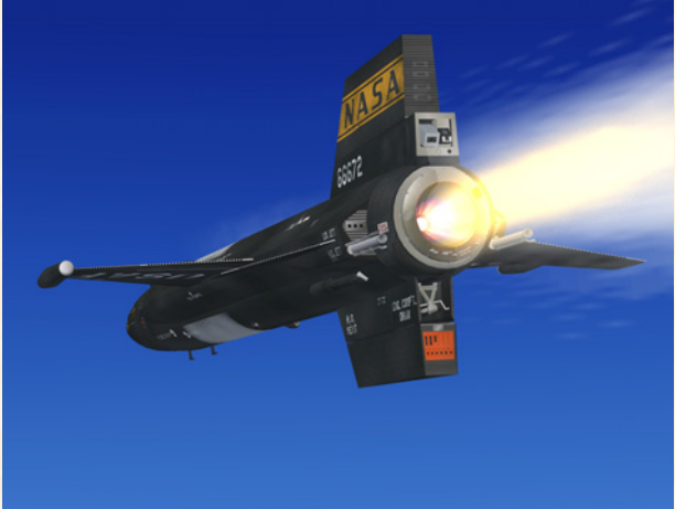
X-15-3 for Flight Simulator. Note the XLR-99 rocket engine and the wing-tip pods. This aircraft also features a tail-cone box containing research instruments.
