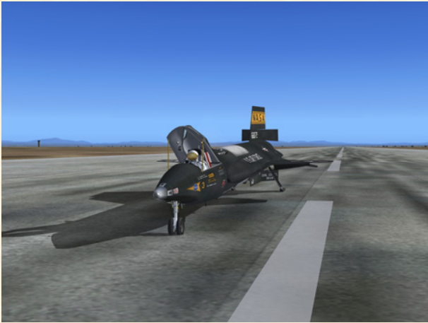
X-15-3 after landing at Edwards Air Force Base. The frost on the fuselage indicates that the liquid oxygen has not been entirely jettisoned before landing and that some quantity is still present in the internal tank. There is no frost on the fuselage when the liquid oxygen tank is empty, on the X-15 for Flight Simulator.
