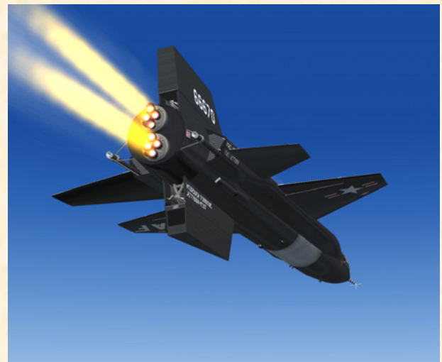
X-15-1 for Flight Simulator in her limited-mission configuration. Note the two XLR-11 rocket engines.
