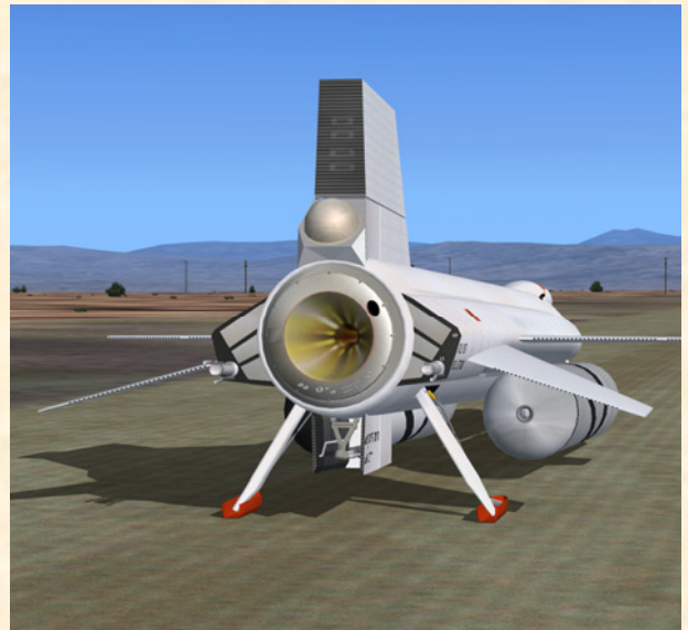
Rear view of the X-15A-2 showing the XLR-99 rocket engine. The dummy ramjet (normally attached to the ventral) does not appear at this time to provide ground clearance and enough space for the rear landing skids.
