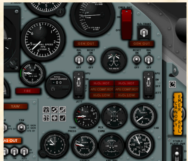
A closer view of the electrical section on the X-15A-2 main instrument panel. Note the APU and generator switches, the dual-pointer AC bus voltmeter and the emergency battery switch.
