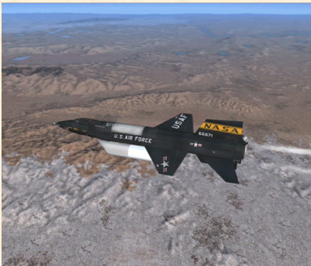
X-15A-2 in flight. Note the frost on the fuselage, around the liquid oxygen tank, and the flow of propellants coming out of the rear prime ports.
