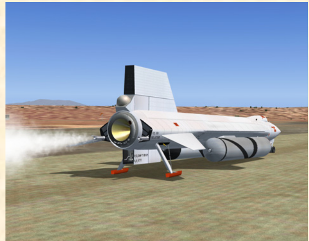
A continuous flow overboard of liquid oxygen vapor is emitted during precooling through the engine liquid oxygen prime valve at the rear of the X-15A-2 aircraft.
