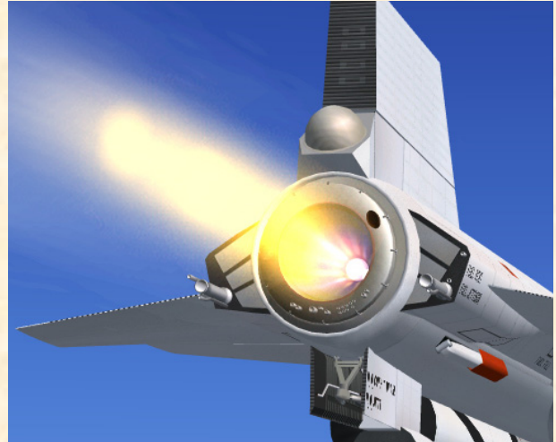
XLR-99 engine start on the X-15A-2 for Flight Simulator. The XLR-99 engine produced nearly 60,000 pounds of thrust at high altitude.
