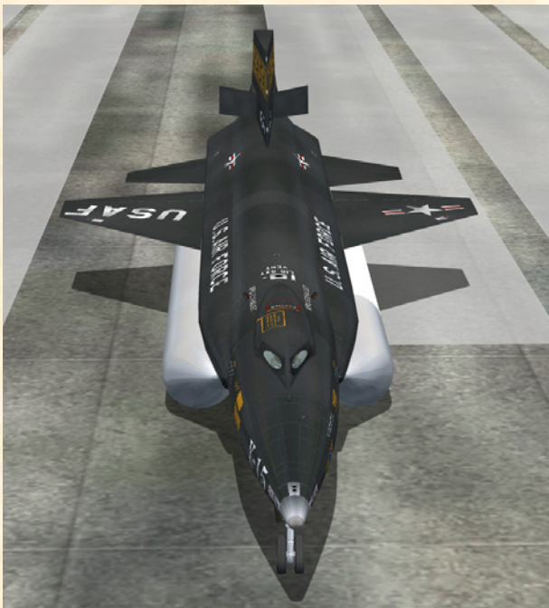
X-15A-2 (rollout version). Note the elliptical canopy windows, the external propellant tanks, a 29-inch fuselage extension (between the internal liquid oxygen and ammonia tanks) and the open speed brakes.
