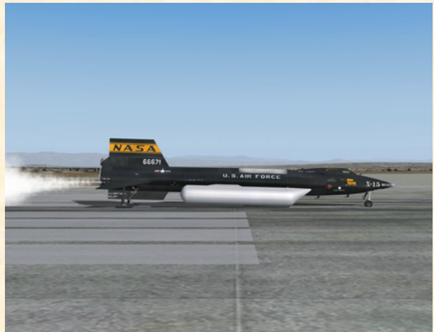
X-15A-2 venting her propellant tanks. Frost and condensation from the cold propellants can be seen on the fuselage and around the internal liquid oxygen tank. The boiling point of liquid oxygen is -297^{\circ} F in standard atmospheric conditions.
