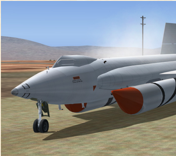
When the APUs are operating, steam should be observed coming out of the APU exhaust pipes.
