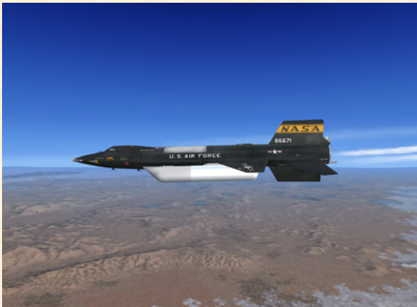
X-15A-2 just before launch. Note the flow of ammonia and liquid oxygen coming out from the back of the aircraft during the engine prime phase.
