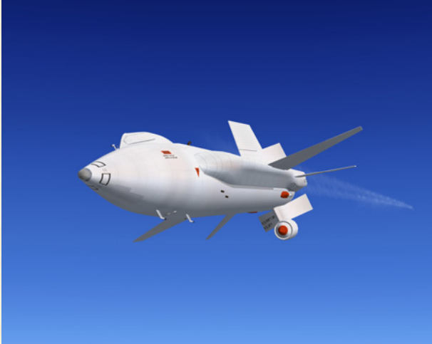
X-15A-2 during her descent and about to perform a 5G pullout to level flight at about 65,000 feet.
