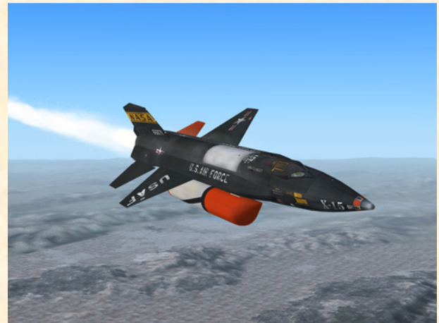
The X-15A-2 for Flight Simulator. The right external tank contains 1053 gallons of anhydrous ammonia and the left tank contains 770 gallons of liquid oxygen.
