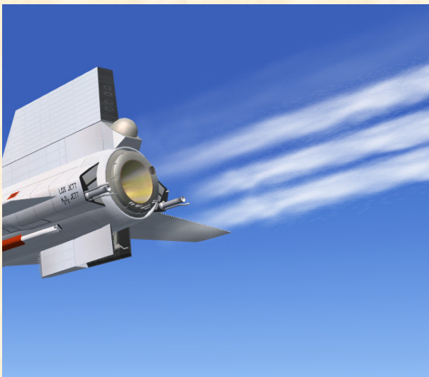
The three propellants (liquid oxygen, ammonia and hydrogen peroxide) are being dumped overboard through the jettison ports at the back of the X-15A-2.
