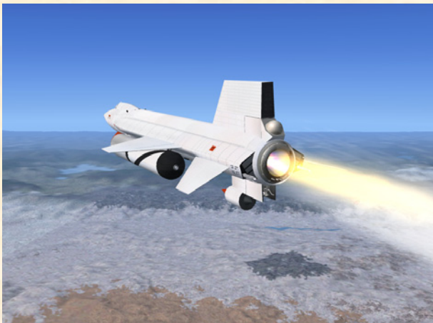
The million-horsepower Reaction Motors XLR-99 engine on the X-15A-2 for Flight Simulator. The XLR-99 was a liquid-fuel turbo-rocket engine of variable-thrust design capable of delivering up to 60,000 pounds of thrust at high altitude.
