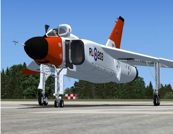
RL-203 before takeoff. Note the open clam-shell canopy and the “vane-type” flight test probe on the nose.
