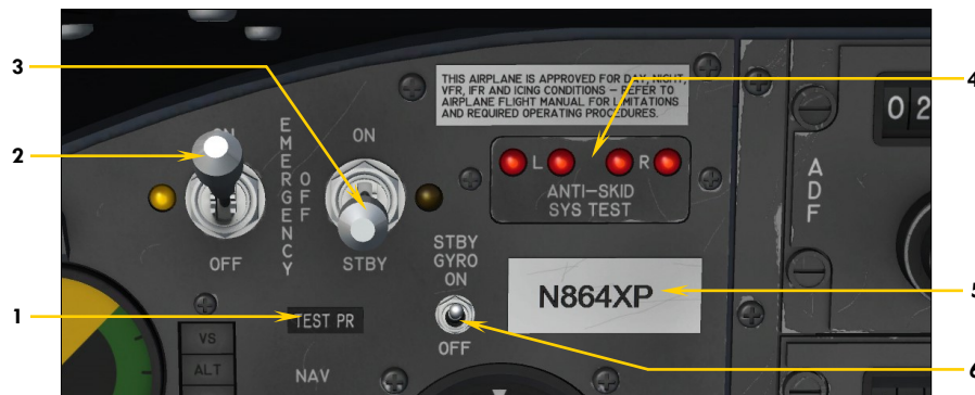
ANTI-SKID CONTROL PANEL Figure 4-15
