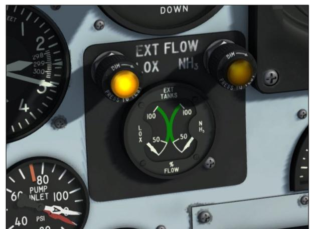
An indication of flow of liquid oxygen and ammonia from the external tanks to their respective internal tanks is displayed in the cockpit on a dual-reading gauge [4, fig. 5-1], on the instrument panel. The gauge is powered by the battery bus.
