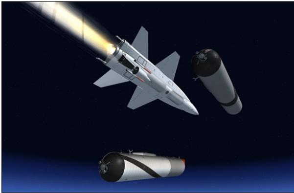
The external tanks must be released before the X-15A-2 reaches Mach 2.6.
