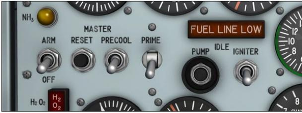
the instrument panel, is powered by the primary DC bus through the engine master switch [63, fig. 5-1]. It has two maintained positions: PRECOOL and OFF (down). With an engine start sequence initiated, moving the switch to **PRECOOL** opens the liquid oxygen main feed valve and precools the system up to the main propellant valve. The precooling flow dumps overboard through the engine liquid oxygen prime valve [4, fig. 3-2].
