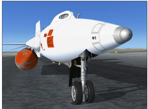
the right on the sideslip indicator. This reading should be maintained for 2 to 3 seconds, then the ball nose should resume normal operation, driving rapidly to indicate the actual angle of attack and sideslip of the airplane.
