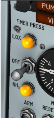
With the switch at **OFF**, the valves are de-energized closed. The switch must be pulled straight out of a detente to move it from **OFF** to either of the other positions.
