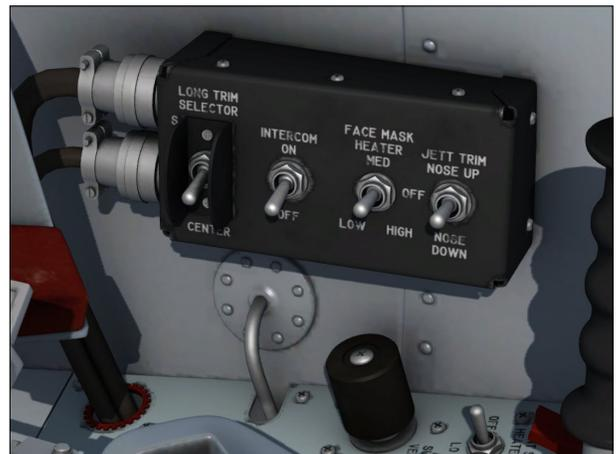
The two-position intercommunication switch [2, figure 5-4], on the left console and labeled "INTERCOM", controls the function of the X-15 pilot's microphone buttons and headset.
