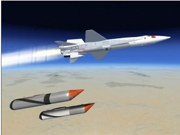
The X-15A-2 SE addon is equipped with two large external aluminum propellant tanks [28, 29, fig. 3-1] to provide a longer engine run which results in added velocity. In flight, the liquid oxygen and ammonia from the external tanks are transferred, under helium pressure, to their respective internal tanks. Indication of propellant flow from the external tanks is displayed to the pilot on the external tanks fuel flow indicator [4, fig. 5-1] on the main instrument panel.
