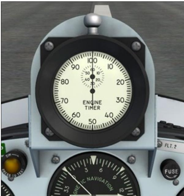
for measuring engine burn time. The timer will start automatically upon ignition of the main thrust chamber and will stop when the engine is shut down. A reset button is provided on top of the timer.
