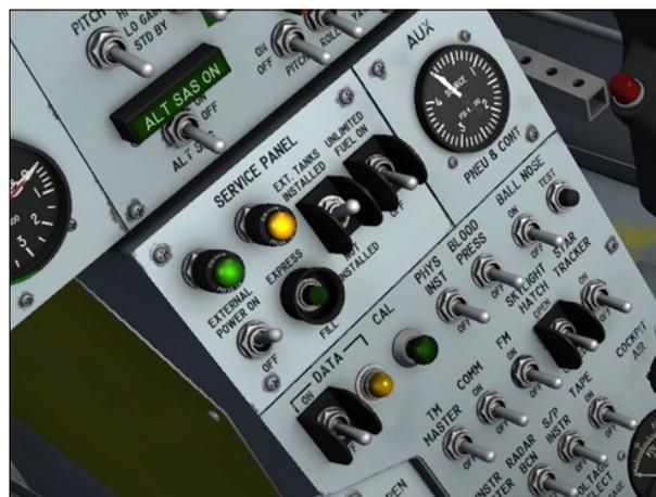
Servicing the X-15A-2 is achieved by the click of a single button on the service panel. The service panel also includes an external power switch to provide electrical power from an external source before takeoff or launch, an external tanks option switch and an unlimited
