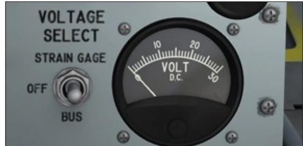
**Note:** Strain gauges (and sensors) are not simulated in this software version. However, the DC voltmeter will indicate 24 volts when the switch is at **STRAIN GAGE**, indicating a normal strain gauge circuit.
