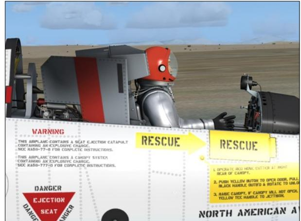
the canopy. Rotating the handle forward and down moves the canopy forward and locks it. Pushing the handle into the spring clip stows the handle.
