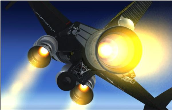
The solid rocket boosters are ignited as soon as the main XLR-99 engine is fired (when moving the throttle [12, fig. 5-4] inboard to **START 50%** at the end of the ignition sequence). They will burn for approximately 50 seconds after which they need to be released either manually or automatically.
