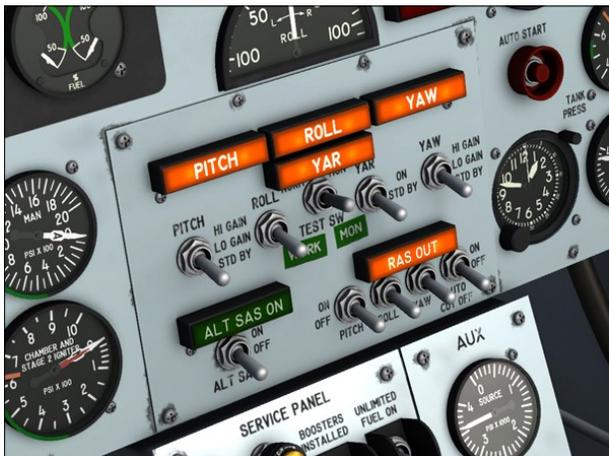
True X-15-type SAS operation is not supported on the current simulation platforms. However, the X-15A-2 SE add-on contains a modified SAS panel [48, fig. 5-1] with the basic autopilot controls for altitude hold, wing leveling, attitude hold and yaw damping modes.
