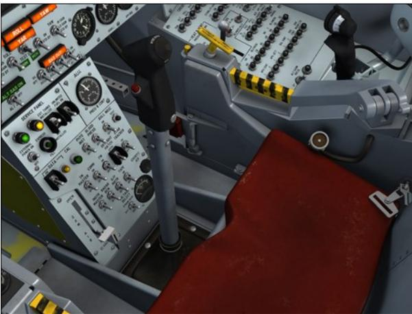
The center stick [8, fig. 4-1] is designed for use during normal periods of longitudinal and vertical acceleration. Pilot pitch and roll inputs to the center stick are summed by the mixer bell cranks and applied to the horizontal stabilizer actuator valves. A microphone button and alternate trim switch are on the stick grip. The button is in parallel with the microphone button on the console stick [3, fig. 5-5].
