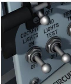
A two-position switch [39, figure 5-1], on the instrument panel right wing, controls the cockpit lighting system. The switch has **ON** and **OFF** positions and is labeled "COCKPIT LIGHTS". The switch is powered by the
