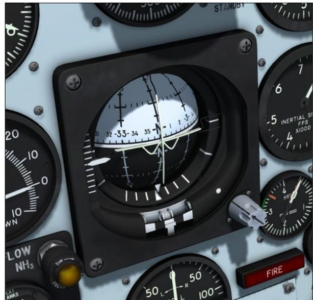
The sphere (remotely controlled by the stable platform) is free to rotate 360 degrees in pitch, roll, and azimuth. The miniature reference airplane is always in proper physical relationship to the simulated earth, horizon, and sky areas of the background sphere.
