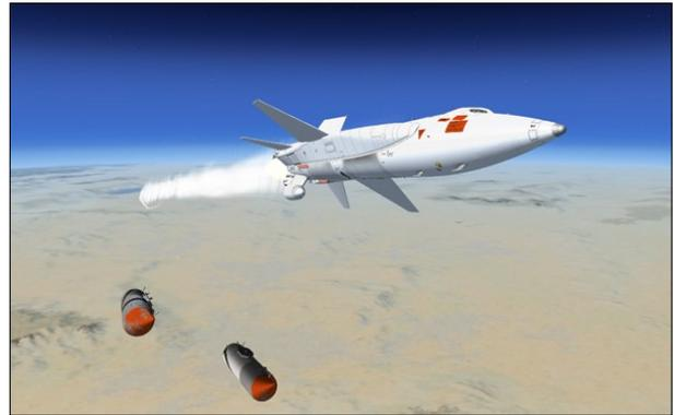
When the external tanks are empty, the system shifts automatically to the internal tanks. Empty, full or partially-full external tanks can be released automatically or manually, as selected by the pilot. Lights in the cockpit indicate when the external tanks are ready to be jettisoned.
