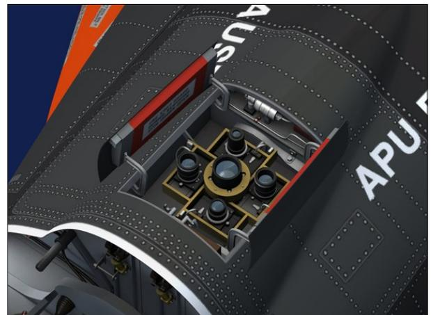
The instrument compartment on the X-15A-2 addon carries an ultraviolet "star tracker" and an ultraviolet horizon scanner that allow for stellar photography experiments. A switch [19, fig. 5-3] on the center pedestal is used to open or close the hatch. An amber caution light [73, fig. 5-1], on the instrument panel, when illuminated, indicates that the hatch is open. For more information, refer to "Instrumentation System Controls and Indicators".
