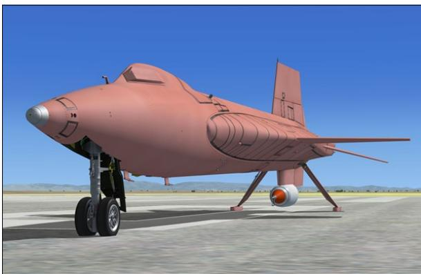
An “eyelid” was designed to protect the left canopy window from being smeared with ablator residue during high speed flight.
