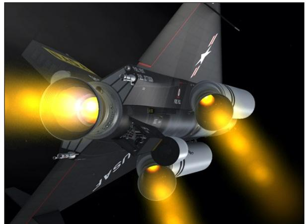
motion by expansion of the combustion gases to a lower pressure and temperature through an exhaust nozzle. The fact that the gases are accelerated by their expansion through the nozzle means that force has been exerted on them to speed them up. The reaction to this force, acting on the forward end of the combustion chamber, gives the engine a forward push.
