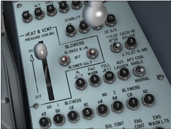
5. Stable platform LN<sub>2</sub> cooling control switch (B-52) - Check **OFF**. Check with launch operator that switch is **OFF**.
