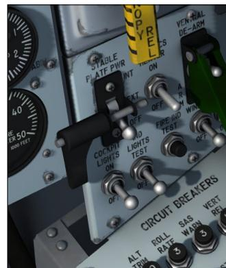
The **OFF** position is a detente position. To move the switch from **OFF**, the switch must be pulled out of the detente. Moving the switch to **INT** energizes the platform with No. 2 primary AC bus power from the APU's of the X-15.
