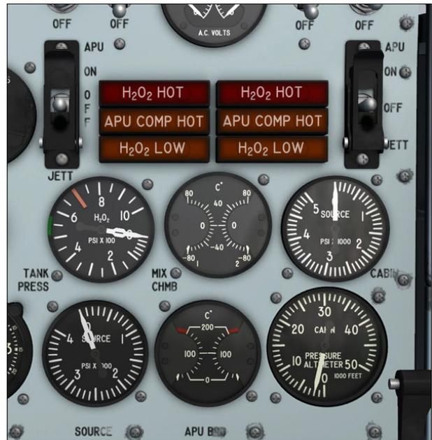
bus power is used to open the helium shutoff valve in the related propellant feed system, allowing helium pressure to move the hydrogen peroxide through the feed lines. At the same time, power is applied to the opening circuit of the related APU shutoff valve. This permits the propellant to flow to the auxiliary power unit.
