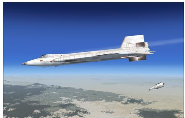
Under normal flight conditions, the dummy ramjet (or ventral) should not be jettisoned except during landing approach. To provide ground clearance for the landing gear, the dummy ramjet (or ventral) must be jettisoned before landing. The dummy ramjet (or ventral) should be jettisoned at an altitude of about 5000 feet and at a minimum of 1500 feet above the ground.
