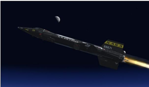
On a real mission, at a Mach number of about 3.0 and an angle-of-attack greater than 10°, the X-15 was uncontrollable without damping when normal piloting techniques were used. The stability augmentation system (SAS) [48, fig. 5-1], installed in the real aircraft, provides damping inputs to the aero-
