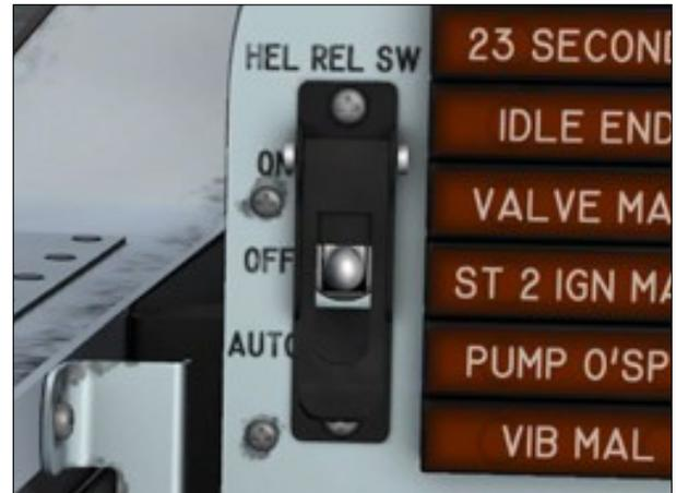
The **AUTO** position sets up an entirely automatic sequence if a fire occurs in the engine compartment, as indicated by illumination of the fire-warning light [47, figure 5-1]. The engine is shut down, and the helium from the two containers outboard of the engine is jet-tisoned into the engine compartment to inhibit the fire or overheat condition and to prevent over-pressurization of the containers by extreme temperature increase.
