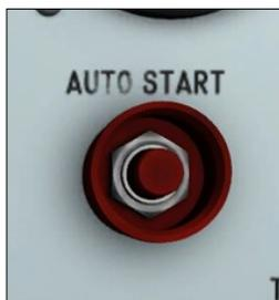
This is similar to pressing "CTRL+E" with conventional aircraft. However, the red button initiates all X-15A-2 rocket aircraft systems, including the special three-propellant fuel management system.
