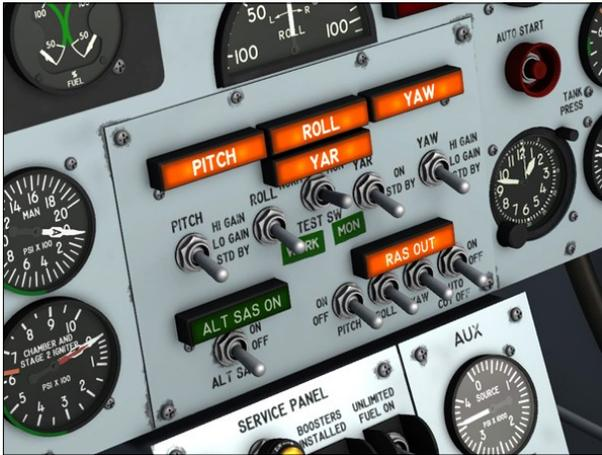
The add-on avionics must be turned on for the basic autopilot to engage:
