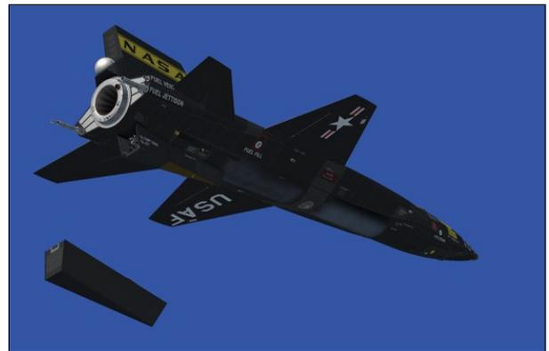
For all flights where the ventral (or dummy ramjet) is installed for launch, the ventral (or ramjet) should not be jettisoned at speeds above 300 knots IAS or Mach 3.5, whichever is lower. Under normal flight conditions, with the SAS functioning properly, the ventral should not be jettisoned except during the landing approach.
