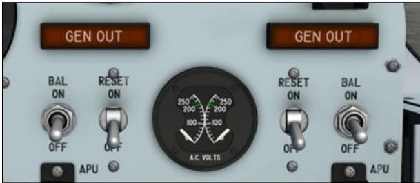
be moved to **RESET** momentarily to bring the generator "on the line" and then released to **ON** to maintain the generator "on the line".
