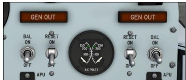
The No. 1 and No. 2 ballistic control switches [18 and 27, fig. 5-1], on the instrument panel, are powered by the primary DC bus.
