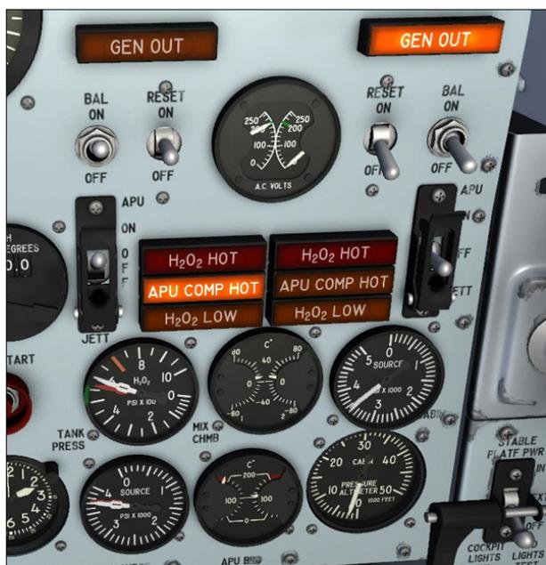
A thermostwitch in each APU accessory drive compartment is set to energize the light when the temperature in the compartment rises to approximately 525° F. The lights read "APU COMP HOT" when on. If either light comes on, the related auxiliary power unit should be shut down immediately.
