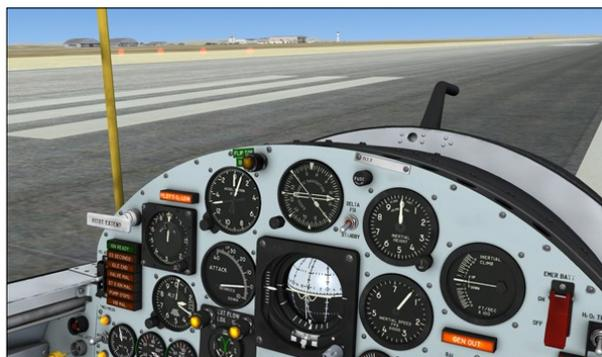
The user can also select whether the engine timer [11, fig. 5-1], located on top of the main panel, is installed or not. This feature may be helpful during landing, especially if the canopy is made invisible.
