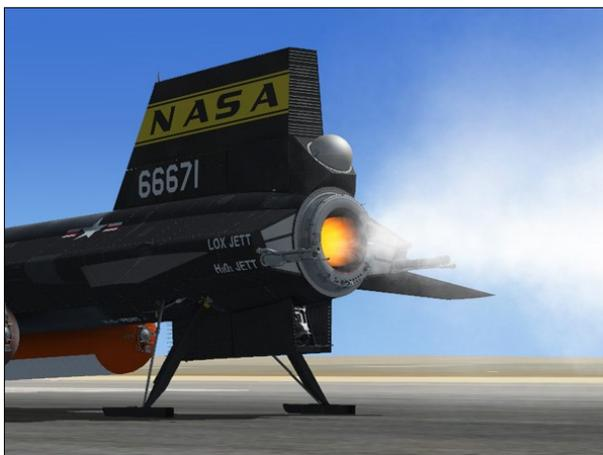
When the main propellant valve opens, fuel and liquid oxygen are injected into the main thrust chamber, where they are ignited by second-stage flames.
