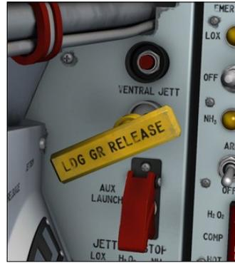
fig. 3-1] uplocks. When the handle is pulled straight aft approximately 11 inches, the uplocks are released, the spring-loaded scoop door [20, fig. 3-1] in the nose gear door swings downward into the airstream,
