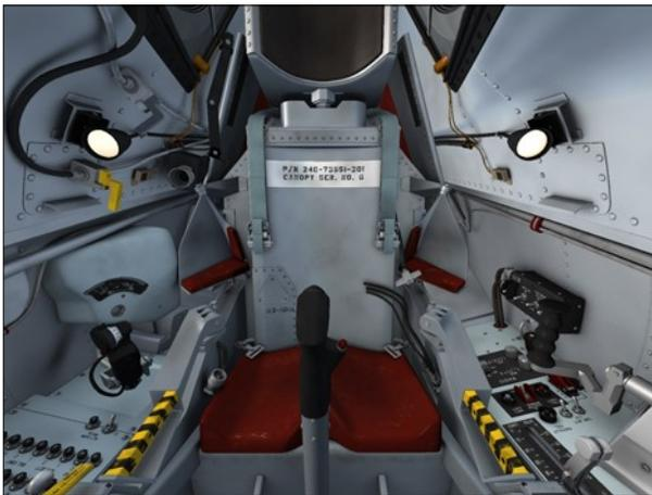
The cockpit is lighted by two floodlights [4, fig. 4-3] attached to the canopy and located so that the light is directed forward and down, covering the entire cockpit controls and gauges. These adjustable lights are shielded to eliminate direct glare to the pilot. A switch on the instrument panel right wing controls the lighting system. The lighting system is powered by the primary DC bus.
