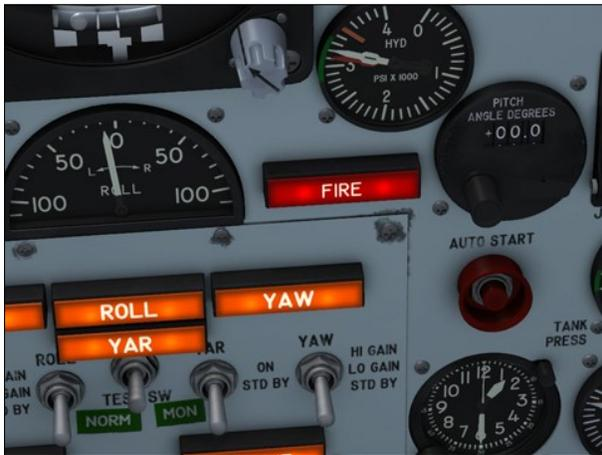
el right wing. The button is powered by the primary DC bus. When the button is pressed, the fire-warning light [47, figure 5-1] should come on, verifying the continuity of the detection circuit.
