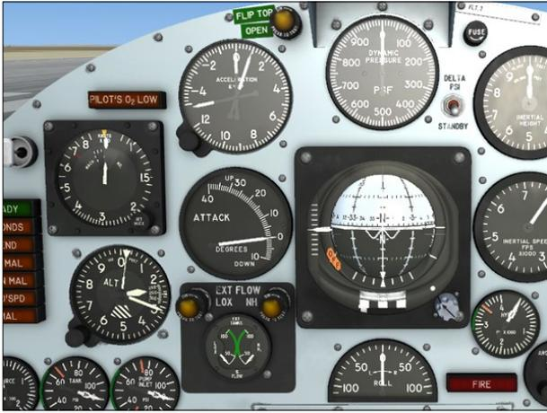
tion forces. Two recording pointers indicate maximum positive and negative G encountered. The recording pointers may be reset by clockwise movement (single mouse click) of the reset knob on the lower left corner of the instrument.
