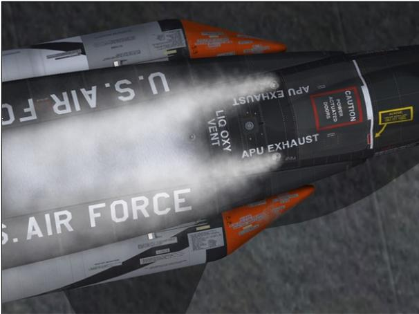
Propellant for each auxiliary power unit is provided by an independent feed system, using helium pressure to move the monopropellant, hydrogen peroxide.
