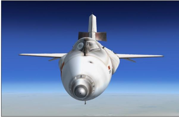
The upper and lower speed brakes must be operated simultaneously and symmetrically. This restriction is imposed because no analysis has been conducted to determine limitations required for asymmetrical operation of the speed brakes.
