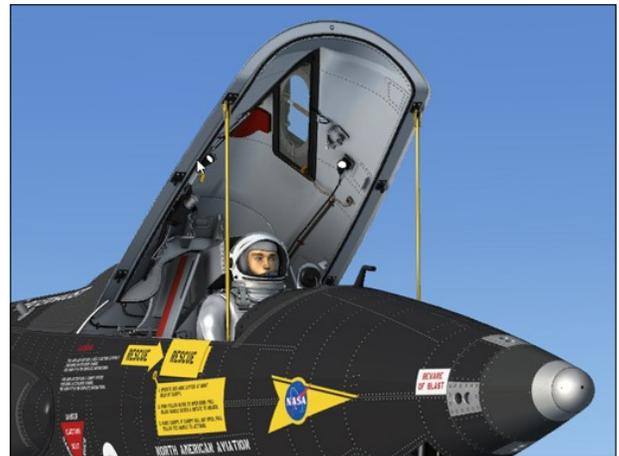
The canopy can also be ejected with the canopy internal emergency jettison "T" handle [32, fig. 5-1] which fires a separate initiator that does not arm and fire the ejection seat when the canopy leaves. A similar "T" handle is provided externally, behind a door [26, fig. 3-1] on the right side of the fuselage, just below the canopy split line, for ground emergencies.
