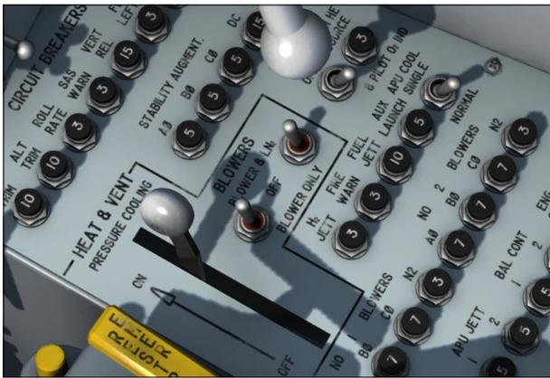
With the switches at **BLOWER ONLY**, electrical power is applied to the blowers, the liquid nitrogen shutoff valves to the injectors are energized closed, and the pressure control valves are de-energized closed.
