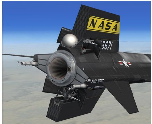
The airplane has two split-flap speed brakes [3 and 34, fig. 3-1], one on the fixed portion of the upper vertical stabilizer and the other on the fixed lower vertical stabilizer.
