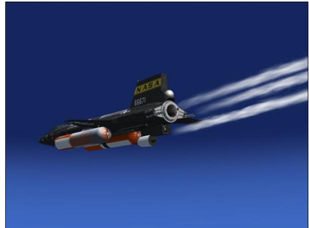
The jettison line of each system should then emit a vaporous cloud. Flow will cease when the switches are returned to the **STOP** position or when the vent, pressurization and jettison control lever is moved to **PRESSURIZE**.
