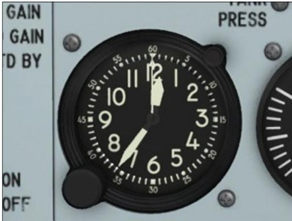
runs for about a week on a single winding. The two large pointers (hands) are the clock's hour and minute indicators. The two small pointers are the stopwatch's minute and second indicators.
